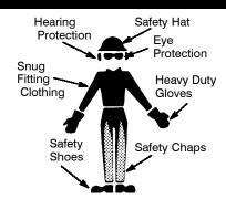
Wear protective gear. Always use steeltoed safety footwear with non-slip soles; snug-fitting clothing; heavy-duty, non-slip gloves; eye protection such as non-fogging, vented goggles or face screen; an approved safety hard hat; and sound barriers (ear plugs or mufflers) to protect your hearing. Regular users should have hearing checked regularly as chain saw noise can damage hearing. Secure hair above shoulder length.
